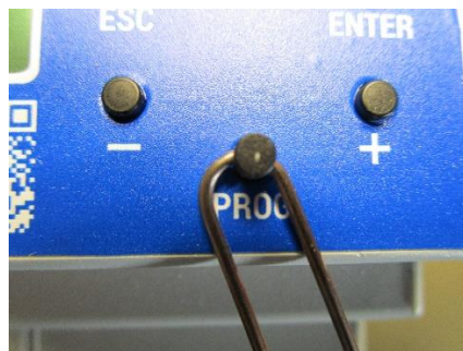
[2.] The sealing wire can be threaded through the hole within this key (max. diameter: see 4.15).
